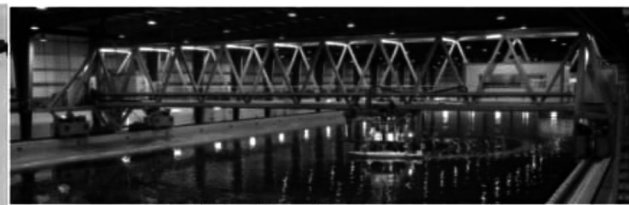
Model testing of a surface vessel
